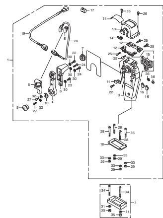
FOP-4-2 REMOTE CONTROL BOX (TOP MOUNT DUAL TYPE) (RIGHT)
